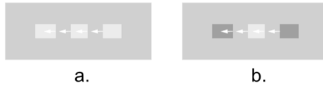
Fig. 6.3. Separated rectangular segments with (a) same luminance contrast polarity and (b) opposite luminance contrast polarity. No real occluder exists between separated segments. The white arrows indicate the terminal edges that are rendered with local motion signals.
